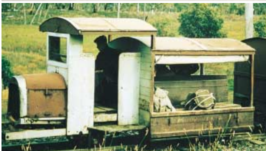
Anti-clockwise, from above: On 9 May 1993, a double-headed tourist train, hauled by Hunslet 0-4-2T No.6 OLD THOMAS and Malcolm Moore 4wDM No.2, crosses the highway at Lune River. Photo: Lindsay Whitham □ The four-wheel petrol railmotor, with trailer attached, used for transporting workers to the quarry, and for carrying bushwalkers to the start of the track to Mt Perouse and all points west, 25 January 1958. Photo: David M Wilson □ The jetty, seen in April 1971, with regular shunting loco No.4, the only Malcolm Moore on the line to be fitted with an open cab. Photo: Frank Stamford □ Malcolm Moore loco No.5 at the Lune River depot in Commonwealth Carbide days. The unusual inertia brakes can be seen on the first wagon. Photo: Tony Coen
