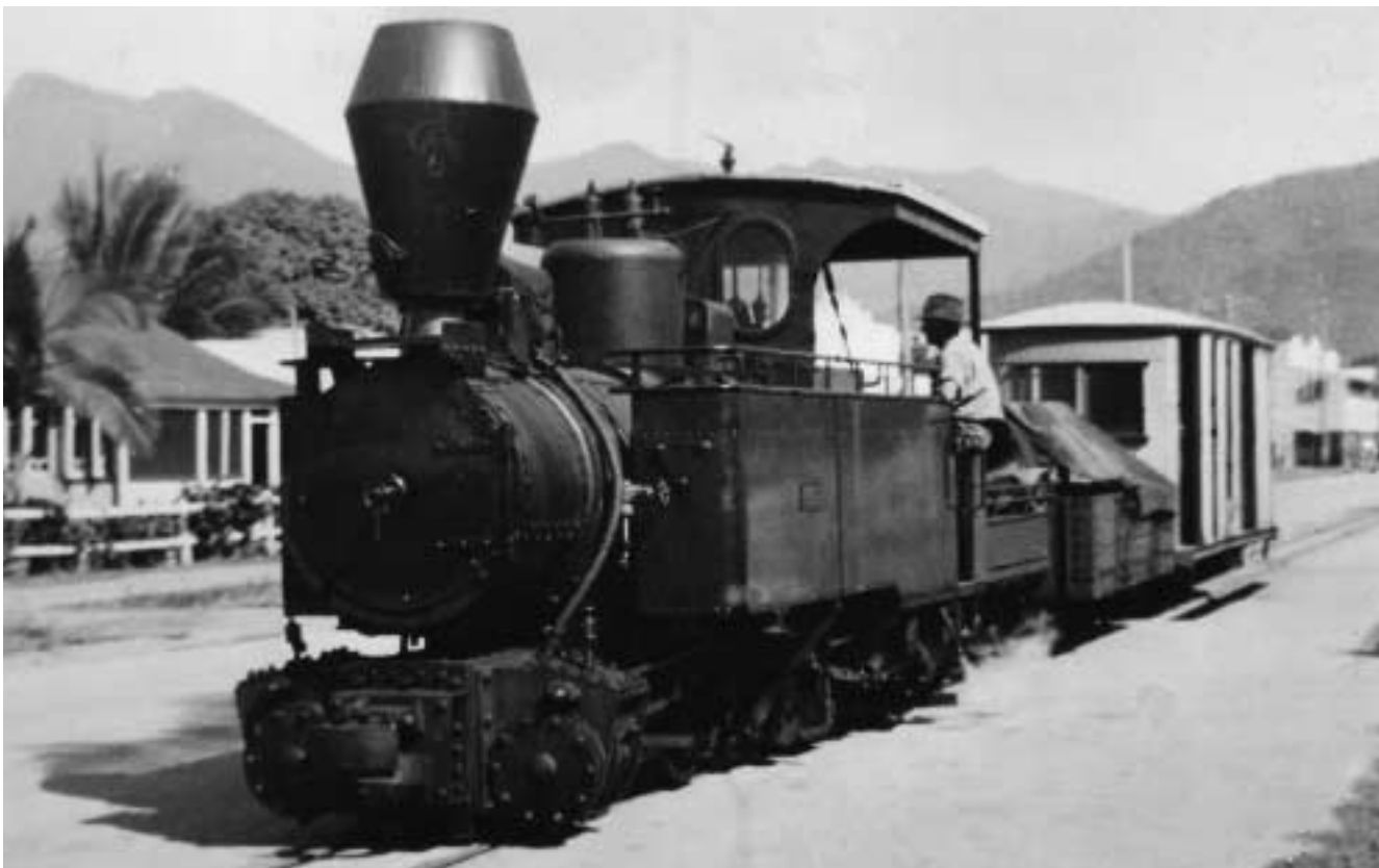
In June 1947, the Mowbray Tram is passing down Mill Street, Mosman, headed by the Shire Council's Orenstein & Koppel 0-4-4-0T compound loco DOUGLAS. (B/N 943 of 1902). Photo: E M Loveday
