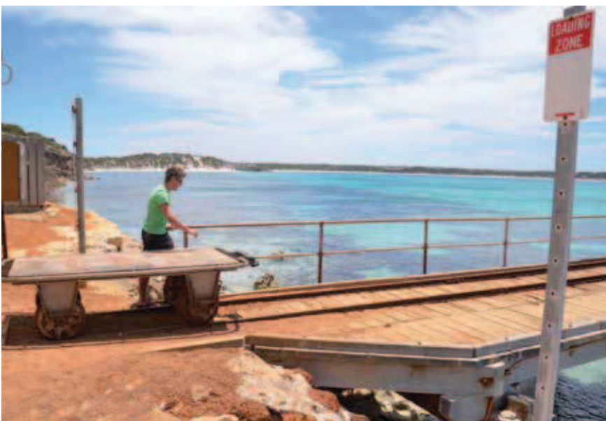
A view of the four-wheel trolley and track at the landward end of the jetty.
