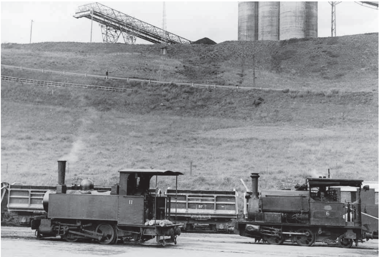
Below: Perry 0-4-0T number 11 (267 of 1926) and Hudswell Clarke 0-4-2ST number 6 (646 of 1903) were both in steam sitting outside the loco shed at the works on 10 September 1966, when an ARE tour was run and six locomotives were in steam for the occasion. Photo: Richard Warren, collection Richard Horne
