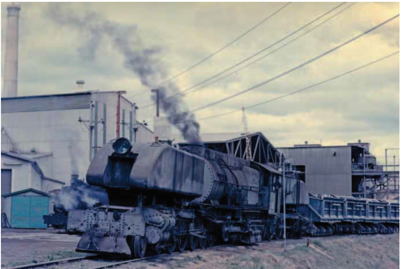
Below: Fyansford's final steam acquisition was this impressive 4-8-2+2-8-4 Australian Standard Garratt (VR Newport 1945), seen here on the loop at the works on 10 June 1966. Photo: Richard Warren, collection Richard Horne
