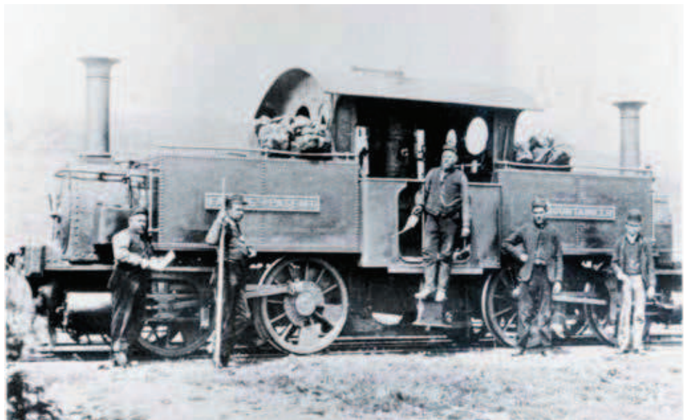
MOUNTAINEER (Fairlie Patent Engine Company 20 of 1869) at work on the Barry Port and Gwendreath Railway in Wales, in 1890. Photo: National Railway Museum Collection
