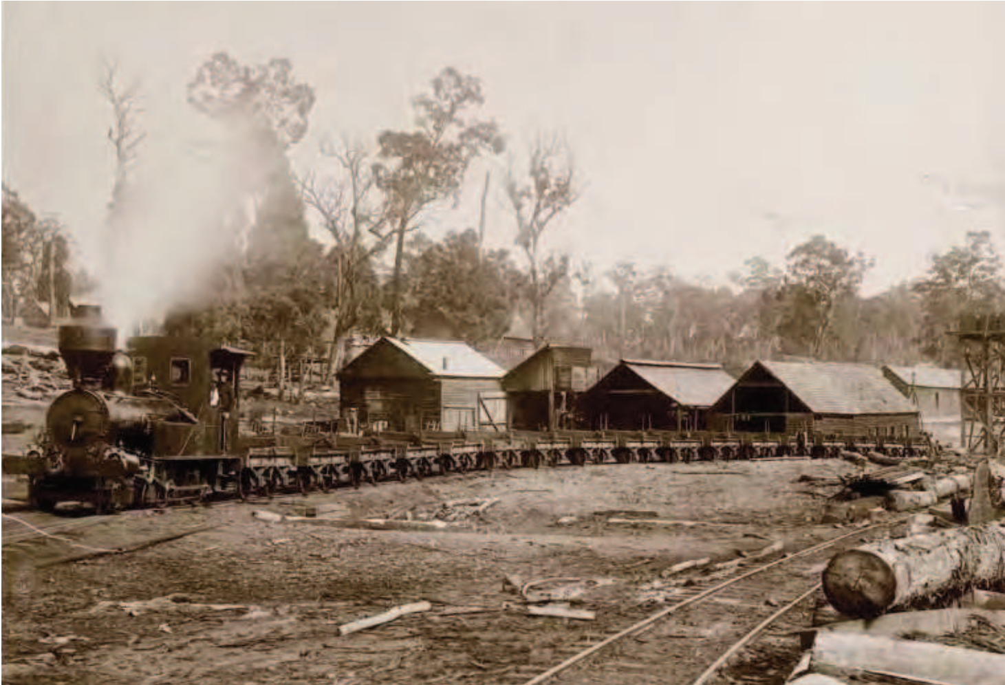
Beyer, Peacock 2-4-0T locomotive SAMSON at Jarrahdale Mill, WA circa 1884-89. Photo: John Ray Collection, courtesy of Bill Weedon
