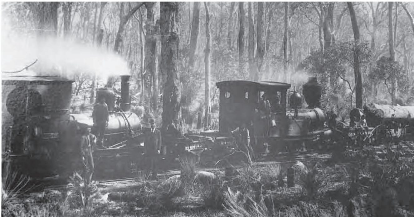
PIIONEER (left) double-heading with one of the SAMSON locomotives. Following the fatal accident of 11 June 1890, PIIONEER was rebuilt with the enclosed steel cab seen here.
