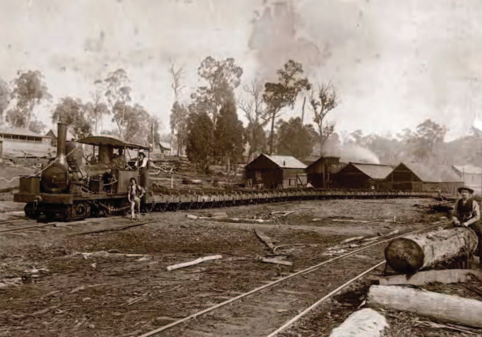
The photograph whose discovery prompted this article. It shows the Fulton Foundry 4-4-0T locomotive PIONEER at Jarrahdale Mill, WA circa 1884-89.
