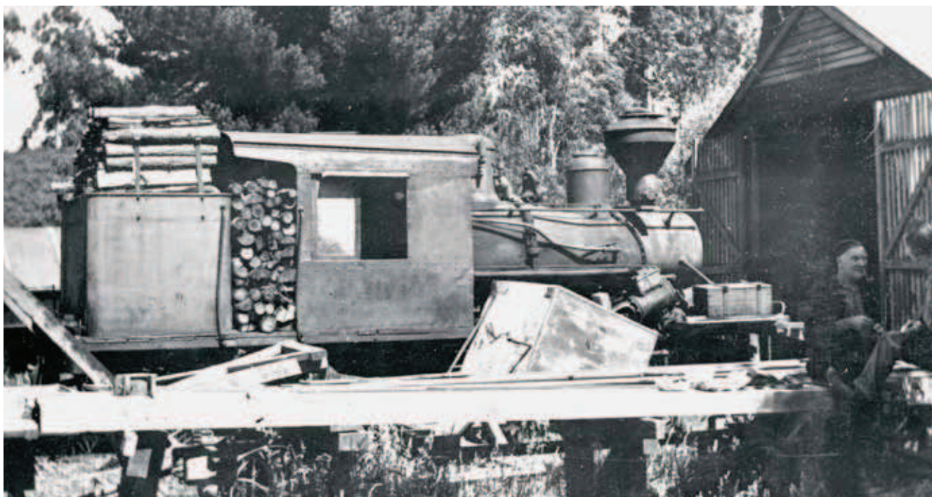
Climax locomotive 1694 at the Tyers Junction loco shed early one morning in 1947, with the cab filled with firewood ready for the day's work.
