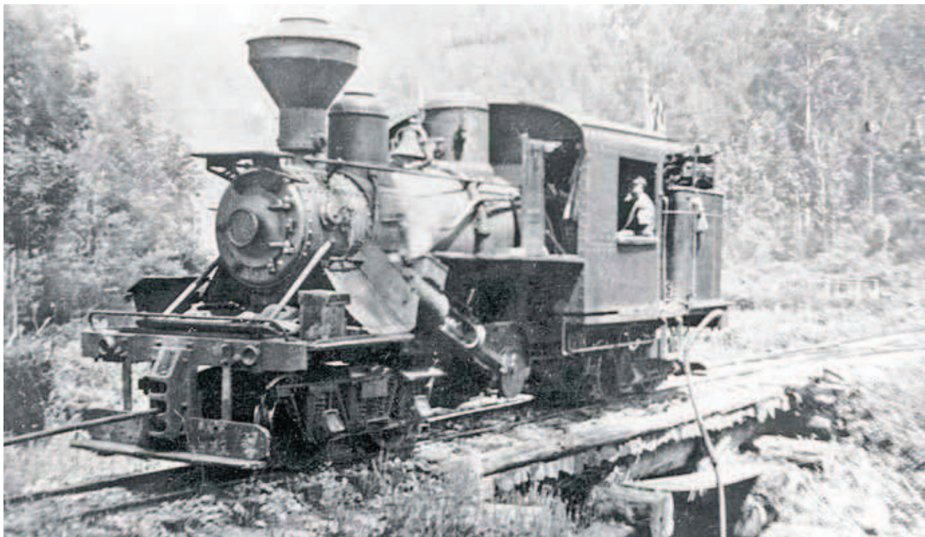
Climax locomotive No.1694 draws water from Hotel Creek, about half-way between Tyers Junction and Collins Siding.
