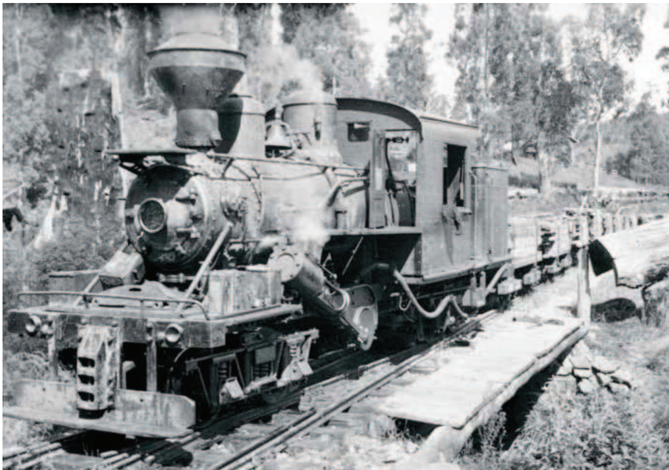
Climax locomotive No.1694 coming into Tyers Junction from West Tyers (on the Ten Acre Block branch). This shows the locomotive with the original riveted smoke box.
