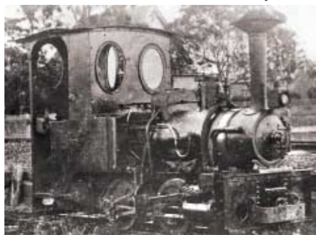
No.2437 whilst working on railway construction in Queensland. Note the square corners on the front plate, and the valve chest set towards the rear of the cylinder block. Photo: Bruce Macdonald collection
