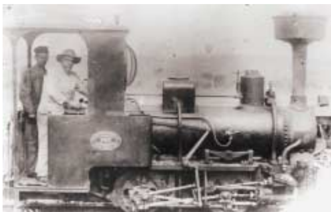
No.2178 working on the Happy Valley project. Note the flat top throttle chamber. Photo: Bruce Macdonald collection
